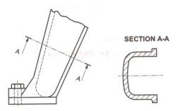
It is similar to revolved type of section except that it does not appear on the view. Here the section is \_\_\_\_\_\_ to some adjacent open place on the drawing. Removed sections of symmetrical parts are placed on the \_\_\_\_\_\_ sion of the center line wherever possible.
